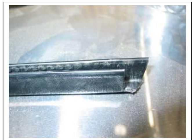
Figure 10. 6mm clip lock trim end trim
