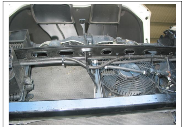
Figure 8: Headlight washer loom attachment under bumper stiffener.
