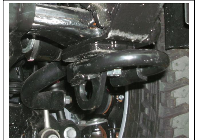
Figure 6: Bolts through tow hook assemblies
